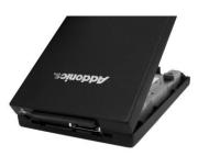
Step 6 Put the top cover on by holding it in near vertical position and sliding the two metal clips inside the two small slots on the rear of the bottom cover.
